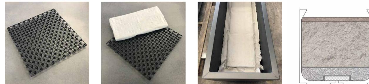
VersiFlex flexible drainage cells are fitted to our large and over-sized pots and planters. These interlocking drainage cells are designed for use in planter boxes, roof gardens and retaining walls. Their open surface design and high internal void volume enable the rapid capture and transport of water volume to result in efficient drainage.
