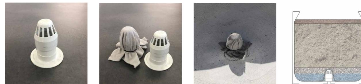
Drainage Regulator Risers are often installed when the amount of water draining from the base of the pot should be limited. They create a 60 mm approx high water reservoir at the base of the pot to prevent excess water from draining away.
