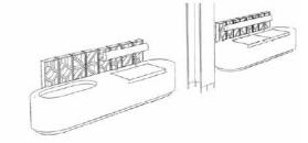
We were able to help the team resolve the furniture designs and provide guidance on the parameters of working with GRC, mould-making and providing block outs for upholstery and the USB charging stations.
