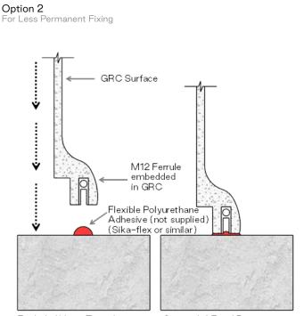
Exploded View: Typical section Secured / Fixed Position CONTACT US
